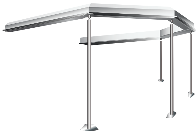
Figure 26: - Example of structural steel posts with ring-beam
