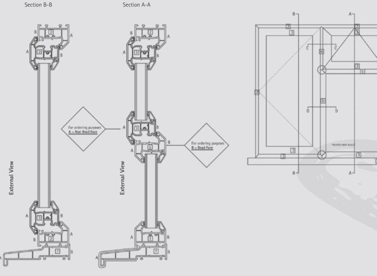
Face A - underbelly of ALL cills to be laminated as shown to ensure continuous colour when viewed from underneath.
