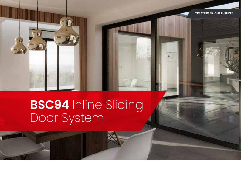
Modern, versatile and customisable, the BSC94 Inline Sliding Door combines high performance with contemporary design to provide a reliable aluminium door system for almost any architectural project. Manufactured to the highest UK standards, this multi-configuration system can achieve thermal U-Values of 1.7W/m²K (triple glazed) and sightlines of as little as 45mm.
